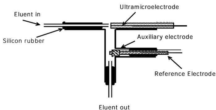
**Figure 1 - Electrochemical cell used in Flow-Injection experiments.**
