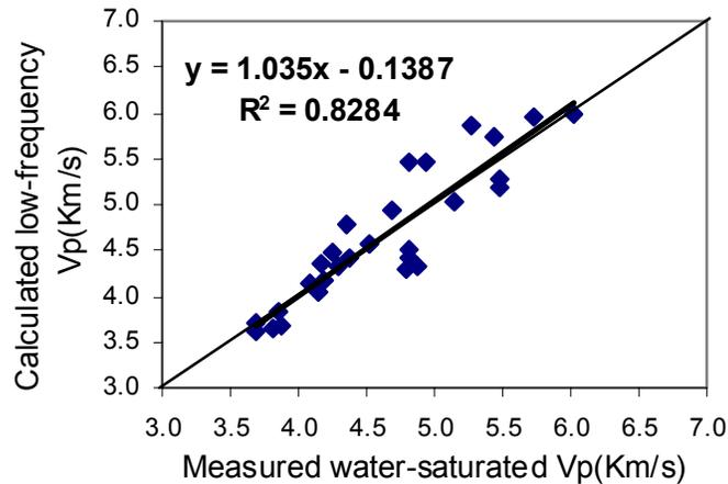
**Figure 2 - Calculated low-frequency Vp using Gassmann's equation versus measured saturated Vp.**
