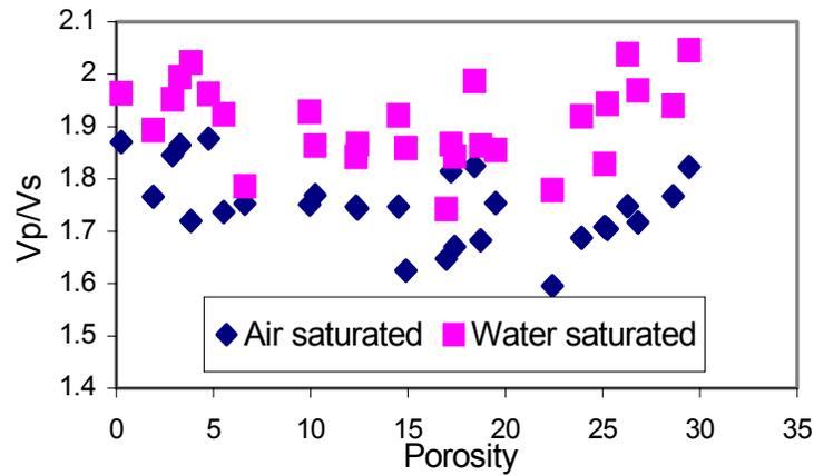
**Figure 5 - Velocity ratio versus porosity at 30Mpa effective stress for air- and water-saturated.**
