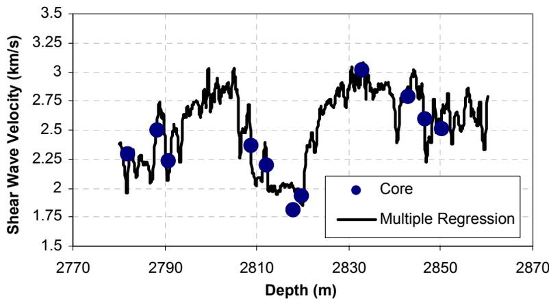
Figure 12 - Core and computed shear wave velocity for well#3.
