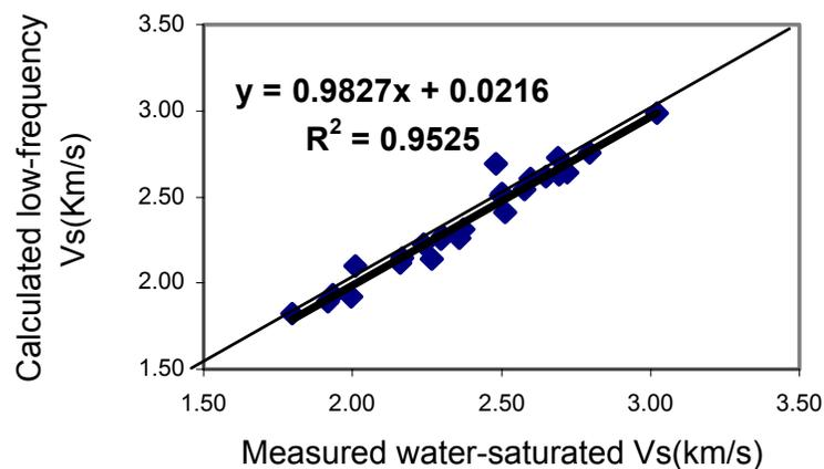
**Figure 3 - Calculated low-frequency Vs using Gassmann's equation versus measured water saturated Vs.**
