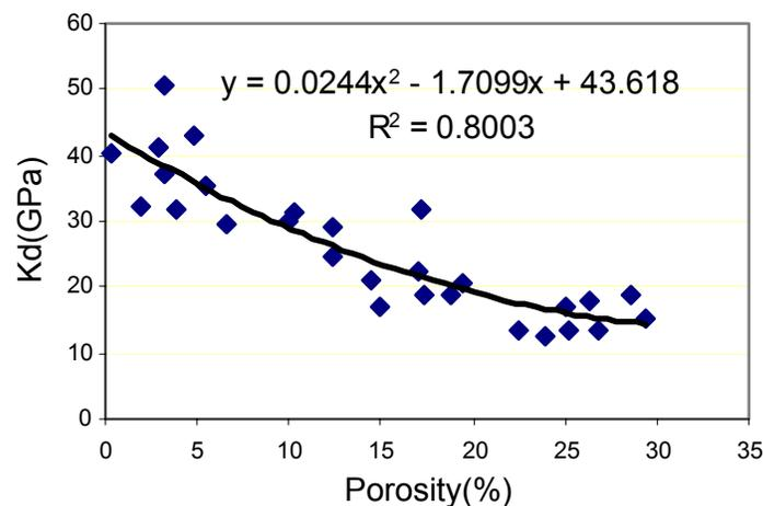
**Figure 1 - Bulk modulus of air-saturated samples versus porosity at 30Mpa confining pressure. At zero porosity,  $k_m$  is equal to 43.618 Gpa.**
