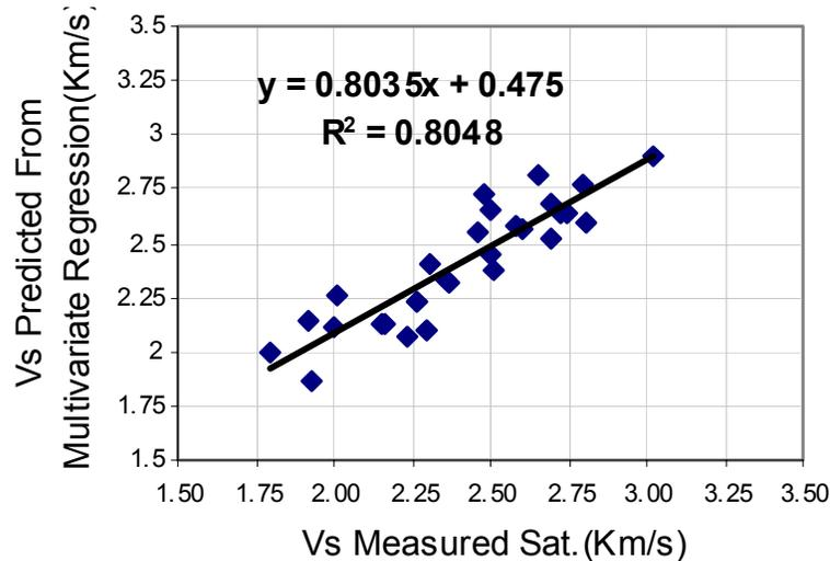
**Figure 7 - Plot of predicted  $V_s$  using equation 8 versus measured  $V_s$  under 30Mpa effective stress and 100% water-saturated condition.**
