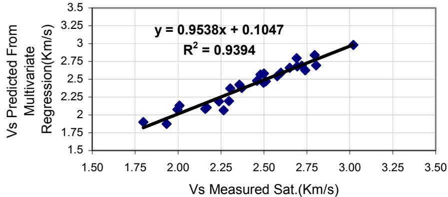
Figure 11 - Plot of predicted shear wave velocity using equation 10 versus measured data under 30Mpa effective stress and 100% water-saturated condition.
